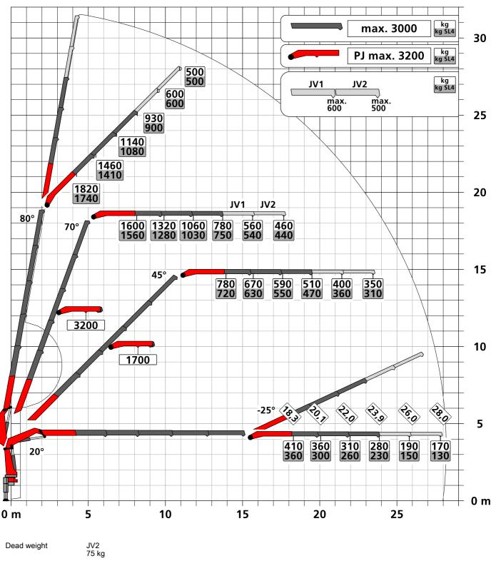
When using mechanical boom extensions, the loads shown on the charts need to be reduced by the weight of these extensions.
