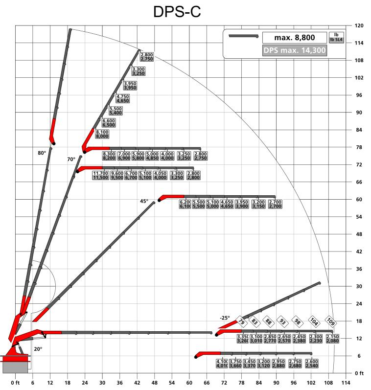
030.01900 Lifting capacity diagram H
