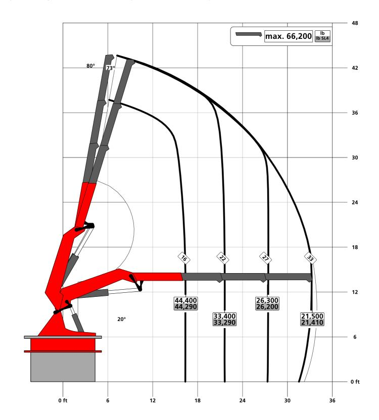
030.01300 Lifting capacity diagram C
