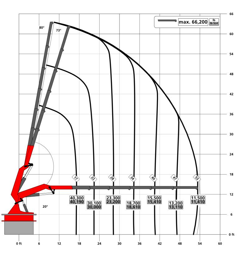
030.01600 Lifting capacity diagram F
