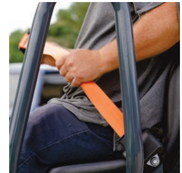
Deluxe seat with high visibility orange seatbelt and integrated side guard
