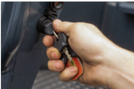
Start the engine with the ground level ignition key
