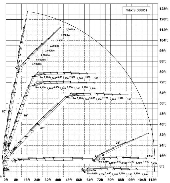
When using mechanical boom extensions, the loads shown on the charts need to be reduced by the weight of these extensions. Symbolic crane figure, indications at 20° main boom position & load arm in horizontal position
