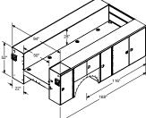
14' standard configuration 52" tall compartment heights 14" tall one handed tailgate Treadplate compartment top overlays
