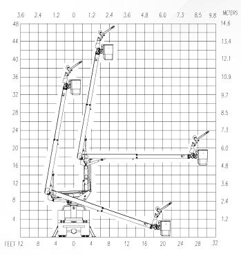
With a 40' working height, 30' side reach, a 24" x 30" bucket, and continuous rotation, the ETC MH 40 IH delivers the maneuverability and reach you expect from a PALIFINGER bucket truck. Single-handle control, basket and turret full-pressure hydraulic controls with complete feathering capabilities, an extended shear ball rotation shaft, replaceable pin bushings, an emergency lowering valve, and engine start/stop at the bucket are powerful standard features
