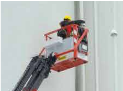
Workman basket Maximised functionality With the aid of the workman basket, additional duties like installation and maintenance work can be performed with the crane.
