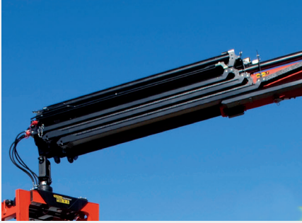
Hose equipment for attachments* Enhances versatility
