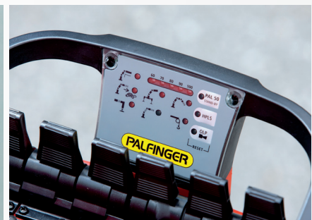
Radio remote control* Dialogue with the operator
