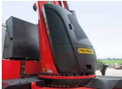
Functional design Practical and attractive Robust plastic covers protect crane parts against dirt and damage. Improved looks and increased operational comfort – throughout the entire lifetime.
