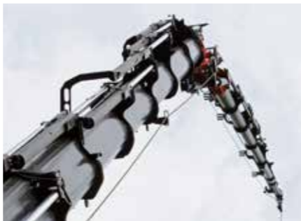
Extension boom system Excellent stability, even at a height Thanks to the use of high-strength fine-grain structural steels in combination with a new extension boom profile, stiffness is increased and weight reduced.
