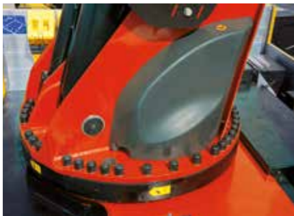
Continuous slewing system Unrestricted movement More efficient in operation due to faster loading cycles, since the crane can be slewed over a shorter distance. The crane works more efficiently and faster.
