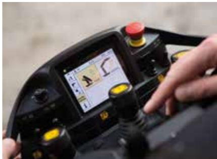
P-FOLD Perfect set-up by fingertip control The new assistance system makes folding and unfolding an easy job for the crane operator. This significantly increases operator comfort and prevents costly damage.
