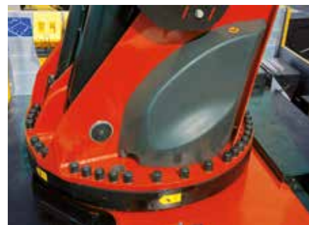
Continuous slewing system Unrestricted movement
