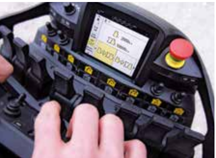
MEXT and WEIGH Systems for easy handling MEXT includes mechanical extensions into the overload protection while WEIGH allows to weigh loads. The result: lower effort for the operator in daily working tasks.
