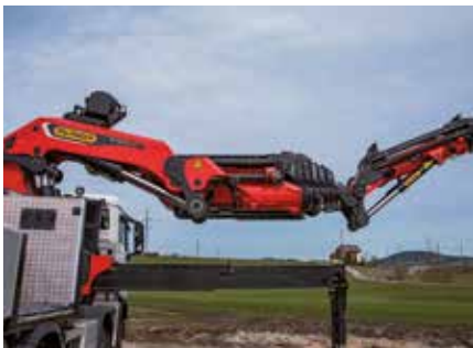
Power Link Plus High variety of uses With the 15 degree reverse linkage system on the knuckle boom and the 25 degree reverse linkage system fly-jib, you can reach through low door openings and also work inside buildings. Heavy crane work – even in difficult conditions.
