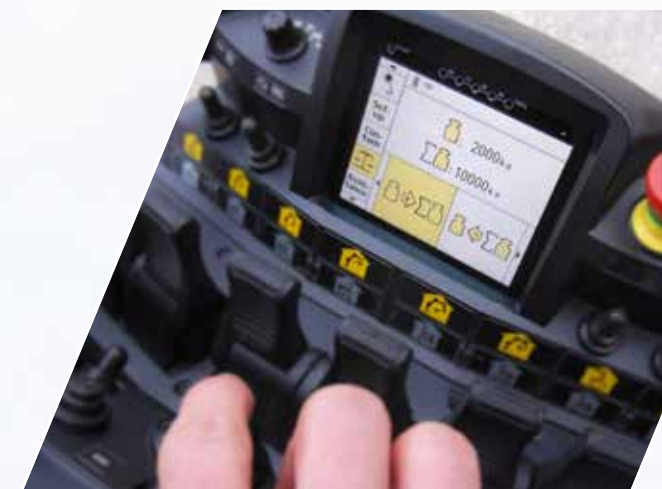
The most recent weigh result is shown above the total weight.
