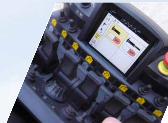
It is possible to integrate one as well as two mechanical extensions into the overload protection.
