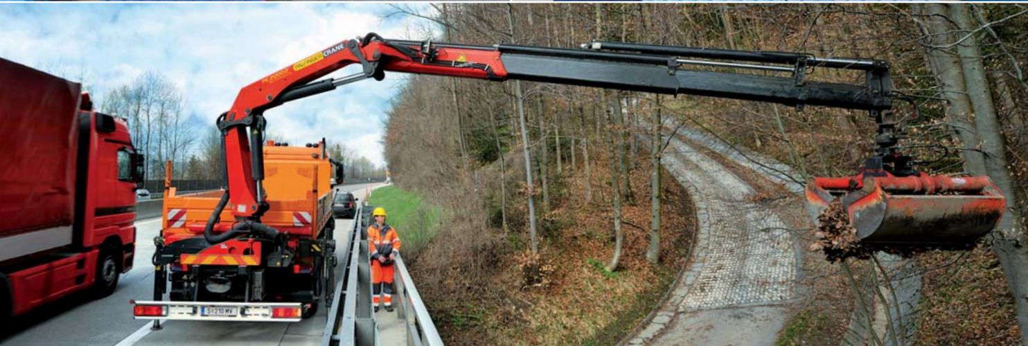
“HPSC” helps the crane operator to achieve maximum comfort and safety even during crane operations where space is restricted. It is often the case in densely built-up areas, in flowing traffic or similar situations that the vehicle can only be supported on one side or it may only be possible to support it partially and sometimes not at all.
