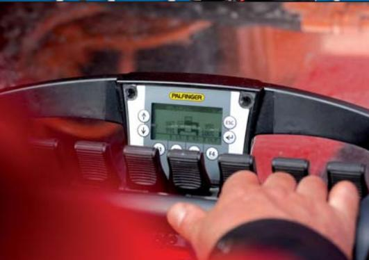
The HPSC system calculates the permissible working range for any slewing angle of the boom system and for any stabilizer situation.
