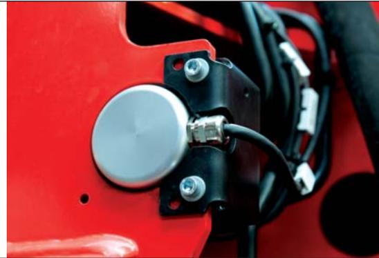
The auxiliary stabilizers are also equipped with proportional length measuring sensors and are integrated in the HPSC. The result is an efficient overall system.
