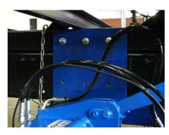
Bolt the console plates to the vehicle chassis. In the process, note the tightening torques in the general installation diagram and in the table on page 29.
