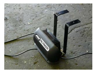
► Fix the control panel holder with screws or weld it in position as per the **PALFINGER Tail Lifts** installation diagram.
