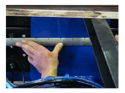
Mark the following holes on the console plate. Observe the general installation diagram and vehicle manufacturer's box body mounting guidelines. Above all, note the number, position and diameter of drill holes.
