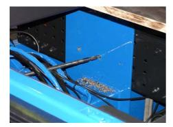
Drill the holes in the console plates.
