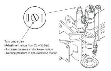
If the hydraulic support raises the vehicle too high or the props do not reach the ground, the pressure switch of the support can be adjusted.
