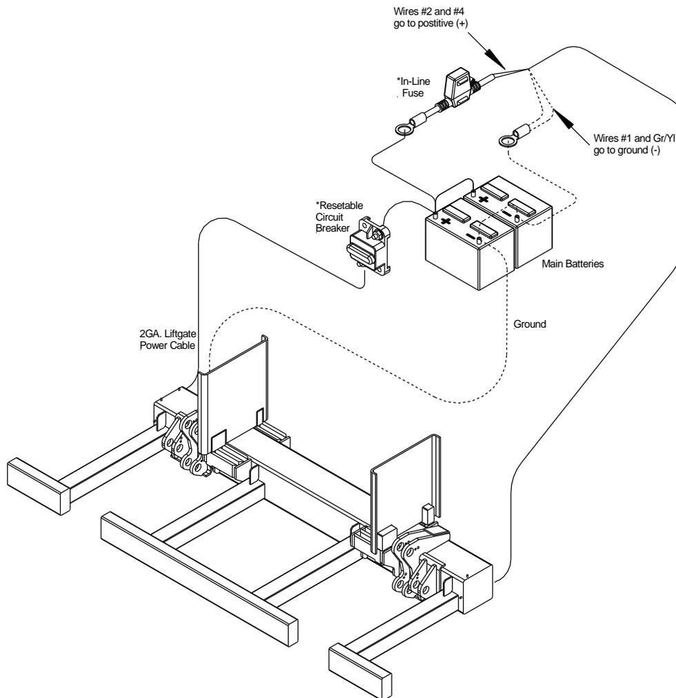
\*In-Line ATC Fuse: 20 Amp. Replace with same amperage fuse when necessary.
