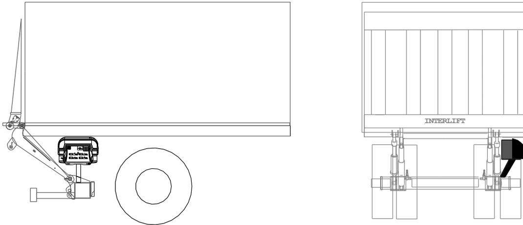
2. Lead the 4-wire cab switch together with the battery cable and the 4 wires for the control power to the batteries along the sub-wood. Secure the cable every 12 inches against the sub-wood with cable staples. Run only the cab switch into the cab. Battery cable and 4 wire control power cable will go directly to the truck battery. (#2 and #4 go to positive post **with an inline 20 amp fuse**; #1 and green/yellow go to negative post)
