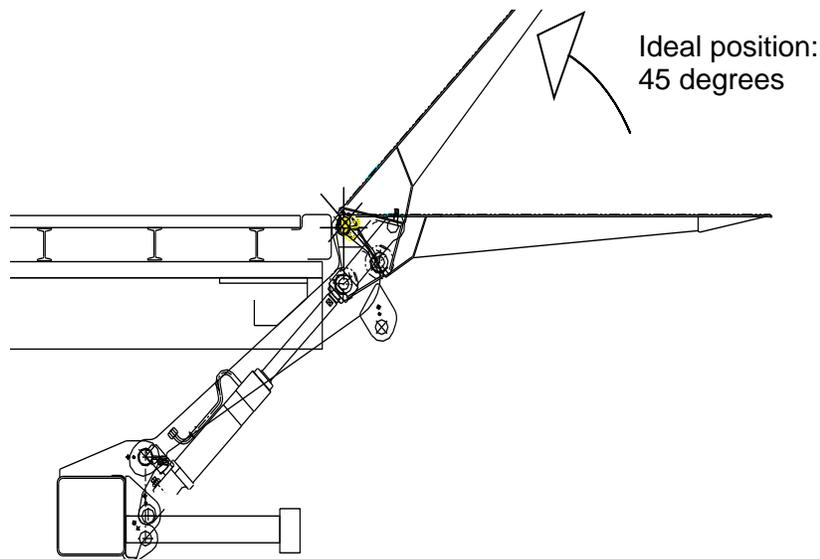
1. Tilt platform up to a point of easy access of the tilt bushings (using the forklift, overhead crane, etc.)
