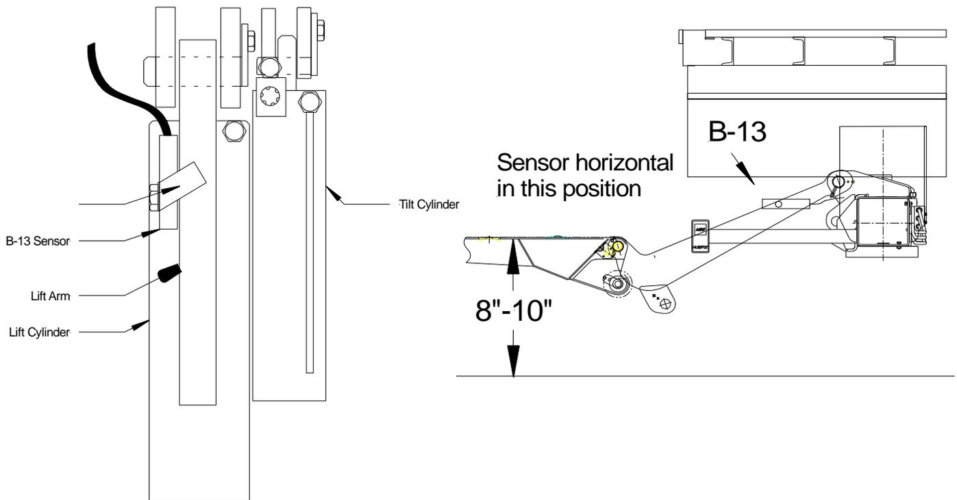
**⚠ At NO time should the platform tilt towards ground while lowering. Platform should ONLY tilt AFTER Lift Arms/Nylon Rollers contact ground.**
