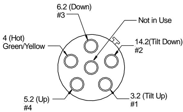
Wiring Socket Connection
