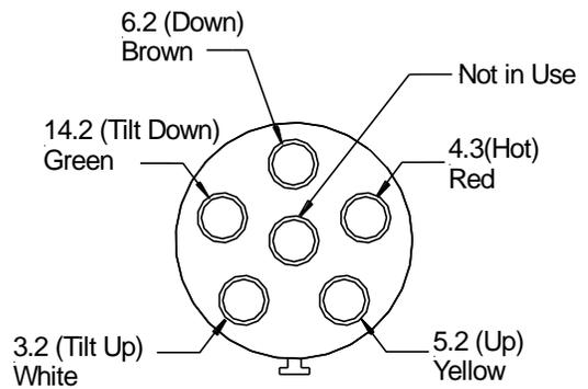
Wiring Plug Connection
