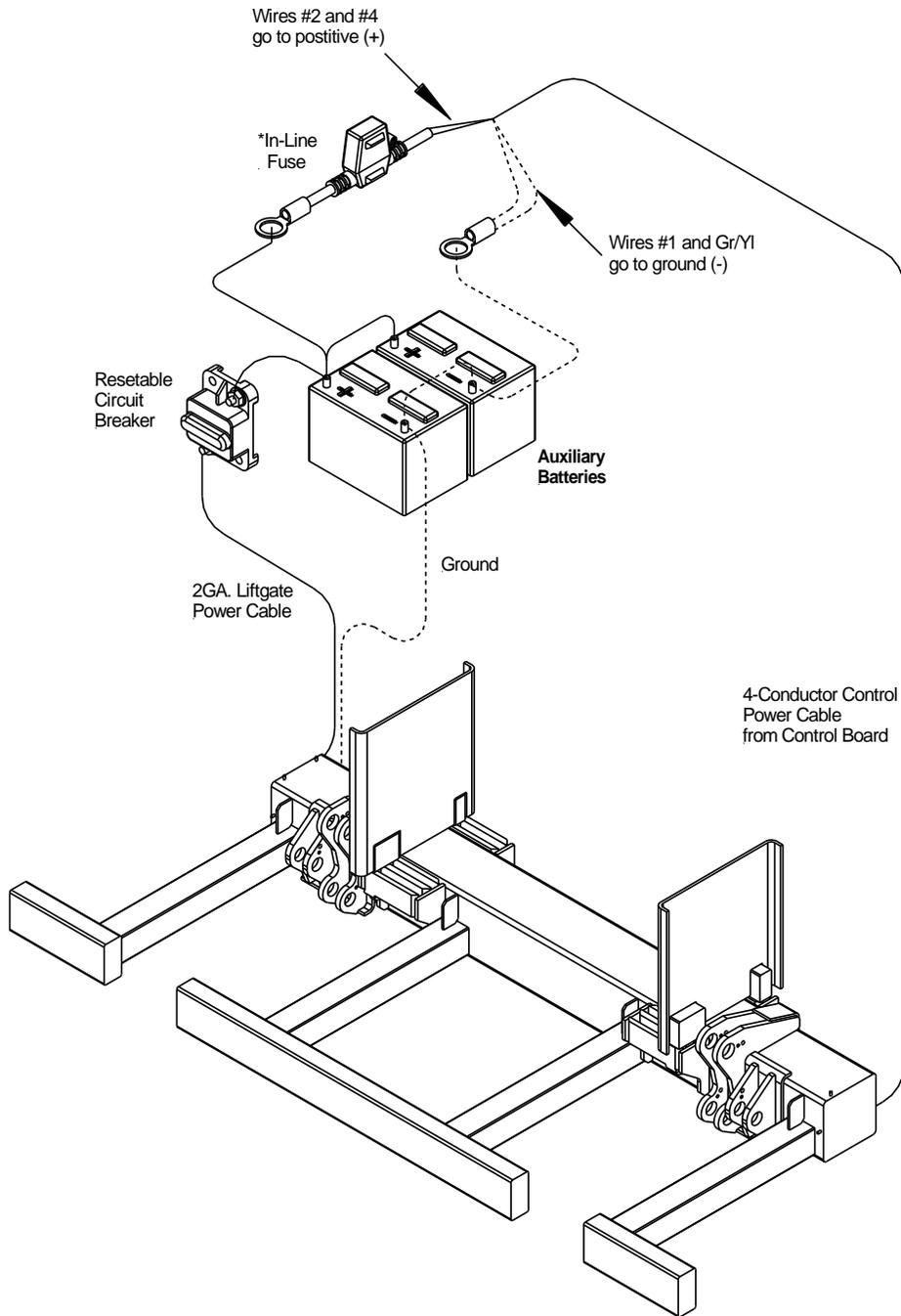
\*In-Line ATC Fuse: 20 Amp. **Replace with same amperage fuse when necessary.**
