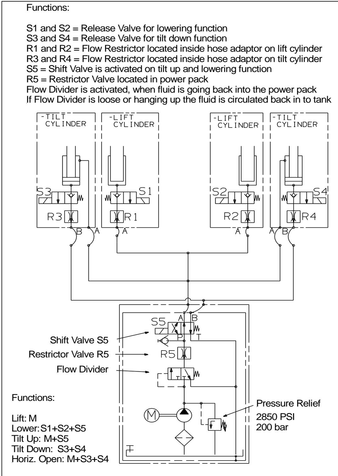
Figure 5.7: Hydraulic schematic
