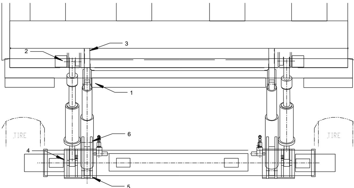
Figure 7.1: Lubrication Points (opposite direction on curb side )
