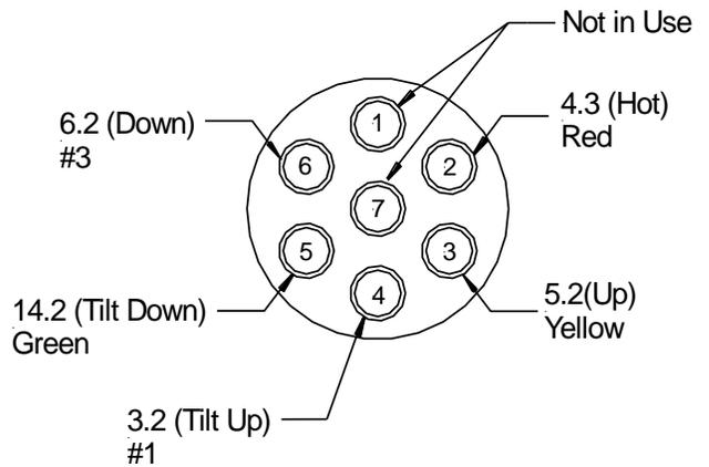
**Wiring Plug Connection
