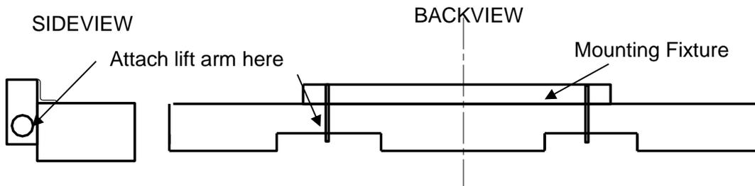
Figure 5.1: Mount fixture welded to rear sill
