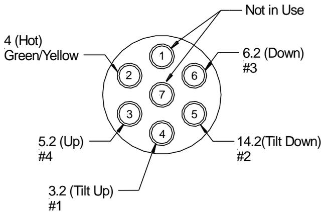
**Wiring Socket Connection
