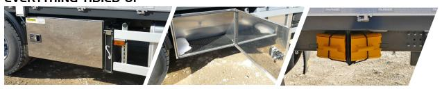
A large stainless steel box is installed on the left and right side. Stabilizer plate holders and wheel chocks are mounted ready to hand.
