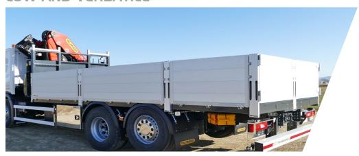
The platform with integrated cutouts for the mudguards is attached laterally to the subframe to keep the loading height as low as possible.
