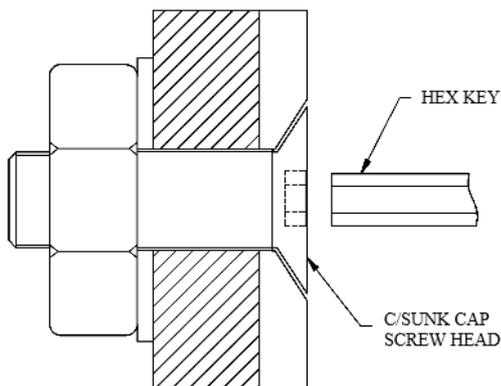
Use a hex key to stop the screw from turning.
