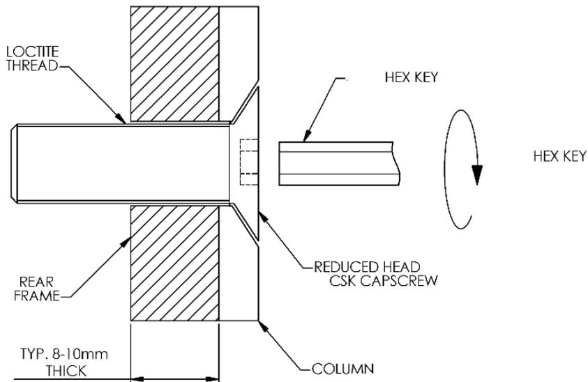
Ensure threads are clean before using Loctite.
