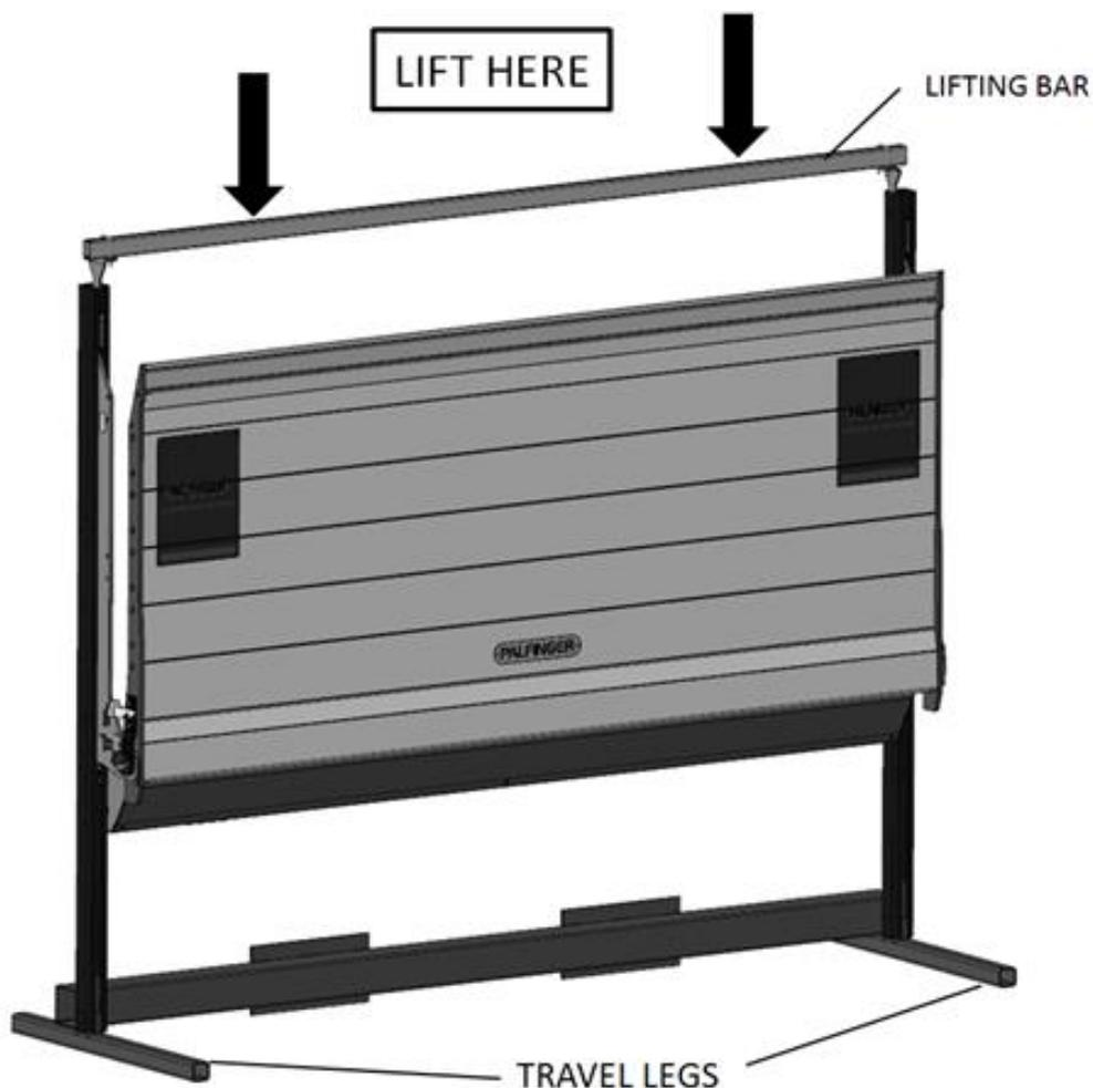
Position the lift so that it is central to vehicle body.
