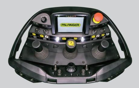
Smart Control enables horizontal or vertical movement of the crane tip with only one lever movement. While the operator only specifies the direction of the crane tip, the electronics (Paltronic) combine the necessary crane movements in the background to achieve exactly the desired position. With a lever movement in two directions, diagonal movements and any curves in space are also possible.
