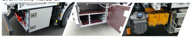
The side walls can be safely stored in the stainless steel box with plywood body at the rear of the vehicle. Stabilizer plate holders and wheel chocks are mounted ready to hand.
