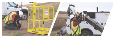
7 REMOVE THE CRANE LOAD BLOCK
