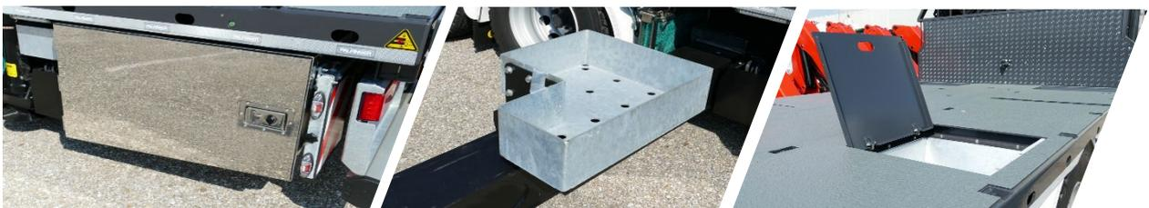
Crane equipment and load handling devices can be safely stored in the stainless steel toolbox with plywood body. Heavy chains are best stowed in the trays on the additional stabilizers or in the boogie trays between the rear axles, where they can simply be picked up with the crane.
