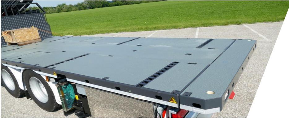
The platform with integrated cutouts for the mudguards is attached laterally to the subframe to keep the loading height as low as possible. The galvanized base coat provides excellent protection against corrosion.
