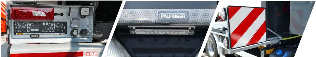
4 LED working lights and 4 LED reversing lights and LED environment lighting provide optimal illumination of the site. Flashing lights at the rear and in the front of the vehicle attract further attention. The extra wide load indicators are equipped with 2 position lamps each side.
