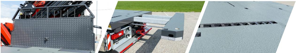
The multifunctional PALFINGER front wall offers a gallery for hanging straps and a coupling for the transport of a trailer. When longer goods are carried the rear can be extended hydraulically by 1m. An anti-slip coating enables safe walking on the platform floor.
