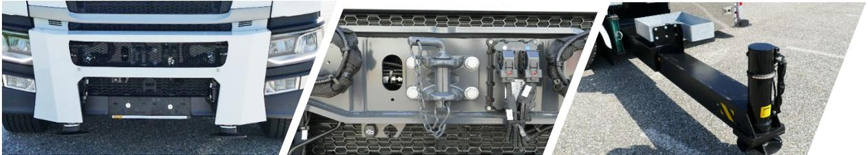
The additional stabilizers and the front stabilizer ensure maximum stability of the vehicle and best crane performance
