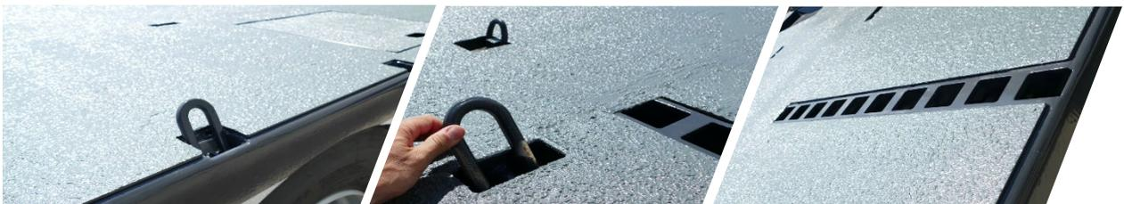
Lashing hooks in the 90° border profile, 10t lashing hooks in the subframe and numerous pole ladders and pole pockets in the platform floor offer the best conditions for the safe transport of heavy and wide goods.
