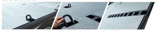
Lashing hooks in the 90° border profile, 10t lashing hooks in the subframe and numerous pole ladders and pole pockets in the platform floor offer the best conditions for the safe transport of heavy and wide goods.
