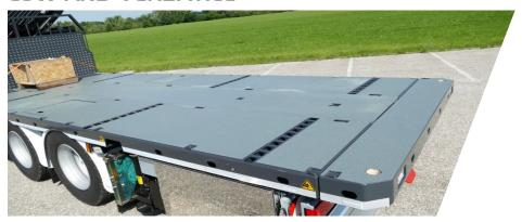
The platform with integrated cutouts for the mudguards is attached laterally to the subframe to keep the loading height as low as possible. The galvanized base coat provides excellent protection against corrosion.
