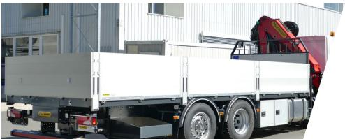
The platform with integrated cutouts for the mudguards is attached laterally to the subframe to keep the loading height as low as possible.
