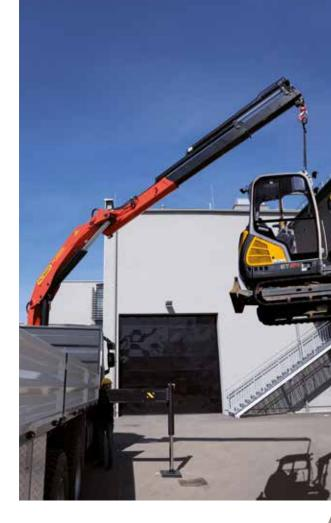
The outreaches stated are with a boom angle of 20° and are therefore not the maximum.
