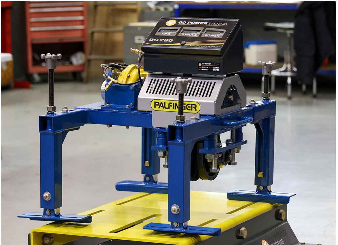
The newly developed PALFINGER Go Power D100LE ("Dyno"), a lifeboat engine dynamometer test stand. © PALFINGER
