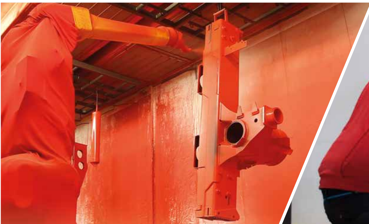
4a.) Top coat with water-soluble and environmentally friendly two component paint
