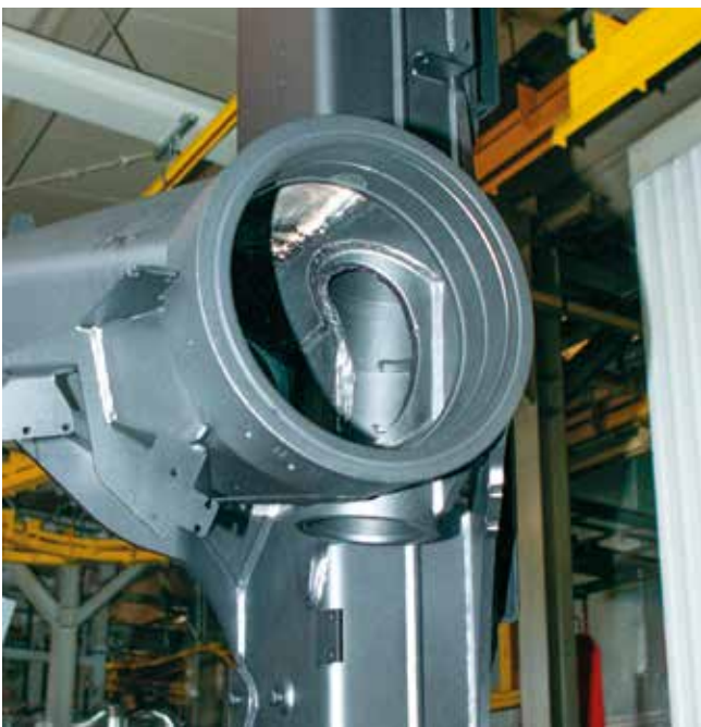
1.) Sand blasted component prepared for the dipping process
