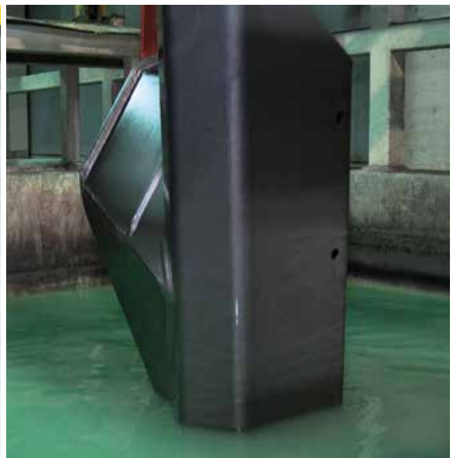
2.) Thorough pretreatment, including high-quality zinc phosphating
